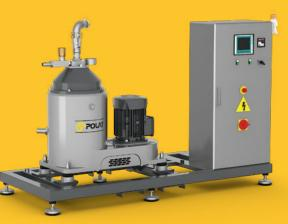
Centrifugal systems operate in by-pass mode with a collecting tank. Experience has shown that good oil quality is obtained if the tank has a capacity equal to 20 times the hourly flow rate of the separator. A purifier separates sludge and water from the oil. Water is continuously discharged from the bowl. The sludge accumulated in the sludge space in both a purifier and a clarifie is intermittently discharged
