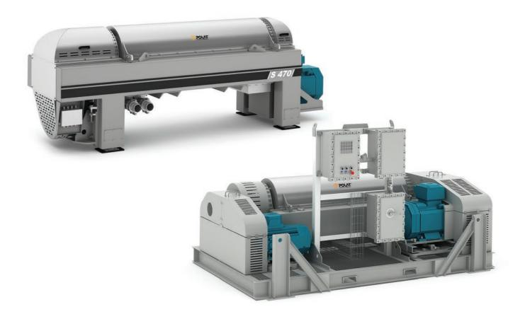
These decanters are designed for feed material which has to be separated into two liquid phases and a solids phase. Separating a feed material into a solid phase and two liquids of different densities in a single operation, with one machine, simplifies the process and reduces equipment costs and space.
