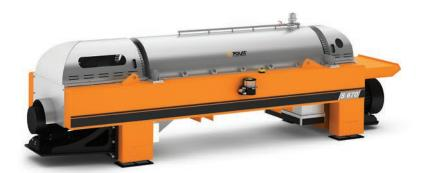
Our **S series** centrifuge decanters are used in the environment, mining, food and industrial sectors. They are designed as a double drive system with VFD. The fully adjustable differential speed of the scroll and adjustable pool depth allow for optimum control of the final product quality.
